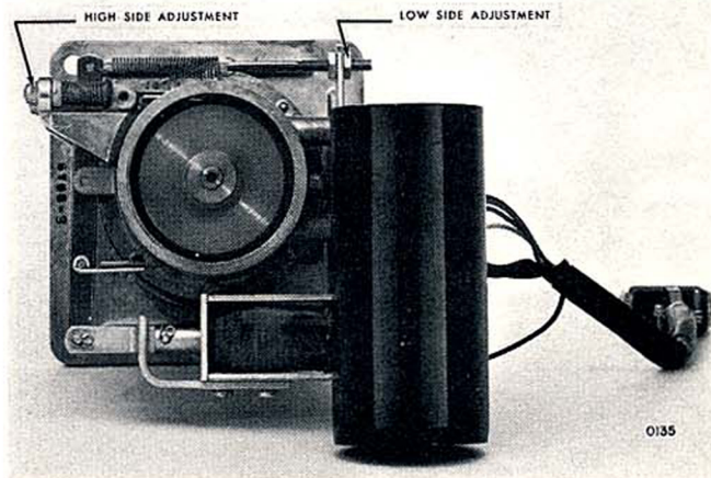
Typical mechanical brake assembly as used by Ampex, showing the two adjustment points.
