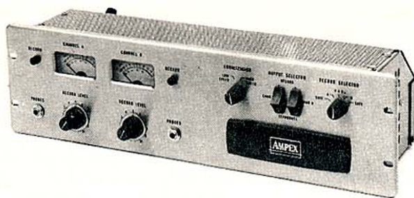
Typical two channel electronic assembly, Ampex Model PR-10-2 professional recorder/reproducer.
