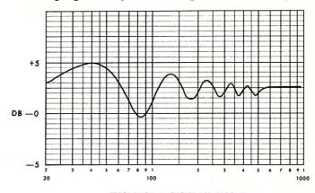
Uncorrected head bump curve produced artificially by excessive tape wrap around an experimental reproduce head.
